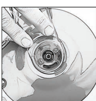
2. Located shield on the Hinge Plate in the closed position
